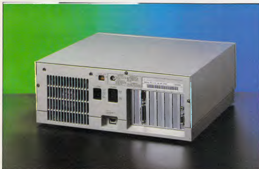
The system box's rear panel is standard PC/AT clone layout
